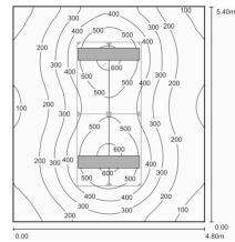
Figure 6: Dialux simulation of the artificial lighting in an aware flexibility concept – level two. Lighting devices simulated are Zumtobel L-FIELDS A A 2/35W T16. Resultat power is 5.83 W/m<sup>2</sup>.
