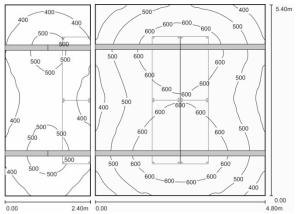
Figure 2: Dialux simulation of the artificial lighting in a full flexibility concept. Lighting devices simulated are Philips TBS340 LC 1xTL-D36W/840 CON C6. Resultant power is 13.12 W/m<sup>2</sup>.
